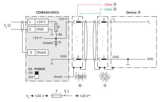
Figure 184: Connecting supply voltage for the device in the CDM420-0001 connection module, Ethernet variant with male connector, M12, 12-pin, A-coded
