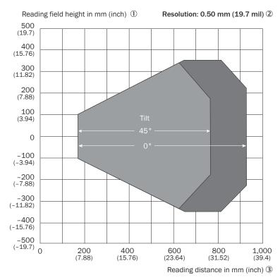
Figure 130: Reading field diagram for CLV651-Xxx0, low density, line (X = 0), glass viewing window, at the front, tilt angle 45° and 0°
