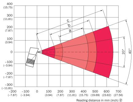
Devices with plastic viewing window (CLV640-6xx1): the depth of field is reduced by approx. 10 %. 3
