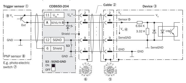
Figure 176: Trigger sensor supplied with power by connection module CDB650-204
