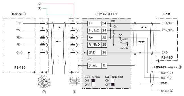
Figure 191: Wiring the RS-485 data interface of the device in the CDM420-0001 connection module, Ethernet variant with male connector, M12, 17-pin, A-coded
