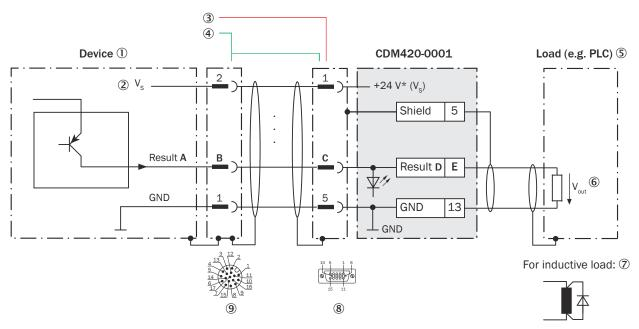
Figure 199: Wiring the "Result 1" and "Result 2" digital outputs of the device in the connection module CDM420-0001, Ethernet variant with male connector, M12, 17-pin, A-coded.
