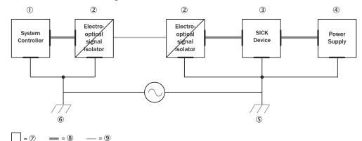
Figure 36: Example: Prevention of equipotential bonding currents in the system configuration by the use of electro-optical signal isolators
