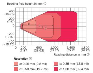
Figure 127: Reading field diagram for CLV650-6xx0, standard density, line with oscillating mirror, glass viewing window, on the side
