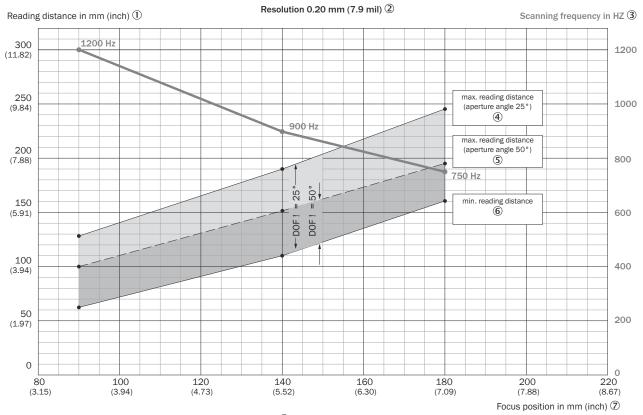
DOF! = xx° D epth of field at aperture angle xx° (8)
