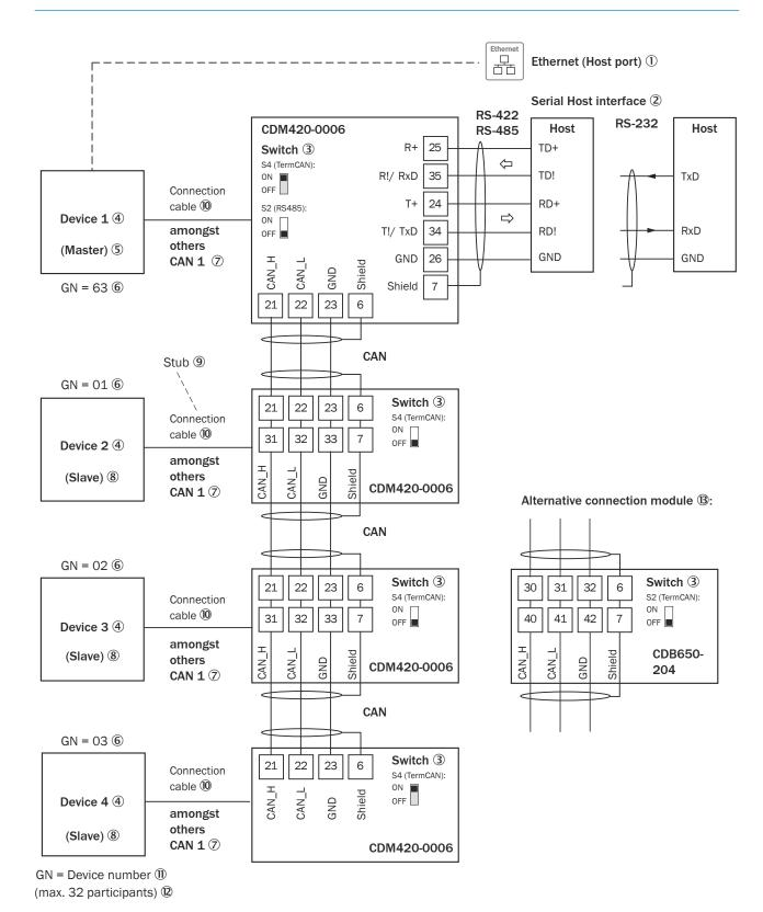
Figure 211: Wire the CAN interface of the device in the CDM420-0006 connection module. Connection and looping through of the supply voltage and connection of a trigger sensor for read cycle generation at the master, for example, are disregarded here!
