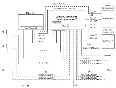
Figure 46: Ethernet variant: Electrical connections on the device with connector (male connector, M12, 12-pin, A-coded)
