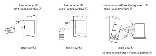
Figure 26: Avoiding surface reflections: Angle between light emitted and bar code (tilting away from vertical)
