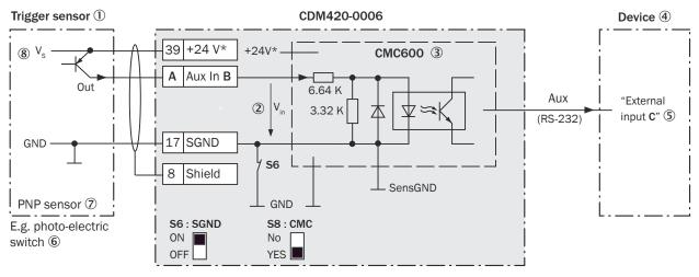
Figure 215: Trigger sensor supplied with power by connection module CDM420-0006.
