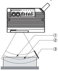
Figure 19: Distance measurement of the device in the IP65 standard housing: Optimizing the depth of field on the object
