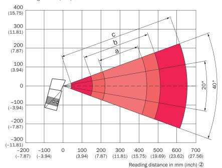
Devices with plastic viewing window: the depth of field is reduced by approx. 10 %. 3
