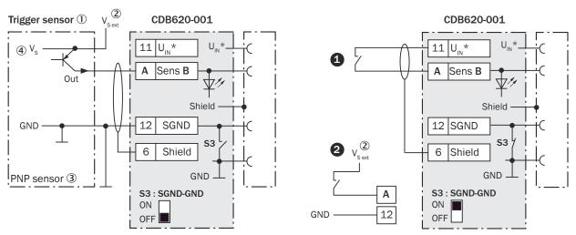
Figure 163: Left: Trigger sensor connected potential-free and supplied with power externally. Right: alternative switch, *1* supplied with power by connection module CDB620-001 or @connected volt-free and supplied with power externally. Now select switch setting S3 as shown in the left figure.
