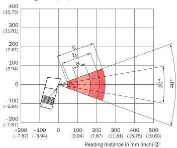
Devices with plastic viewing window (CLV640-6xx1): the depth of field is reduced by approx. 10 %. 3
