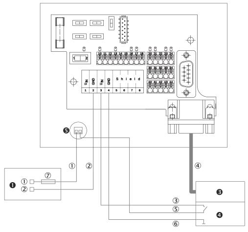
Figure 50: Supply voltage wiring for device and heating in CDB620-001 connection module
