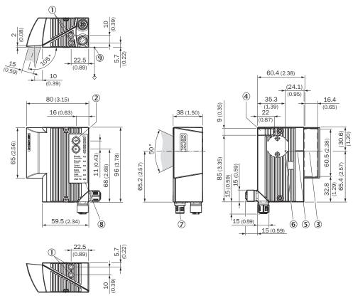
Figure 68: CLV63x to CLV65x: Ethernet variant in standard housing, with side viewing window and swivel connector. structure and device dimensions, unit: mm (inch), decimal separator: period
