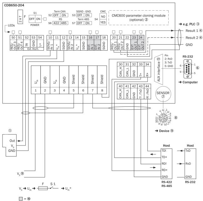
Figure 170: Overview: connection of device and peripherals to the CDB650-204 connection module
