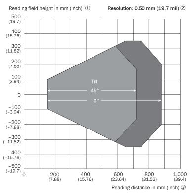
Figure 132: Reading field diagram for CLV651-6xx0, low density, line with oscillating mirror, glass viewing window, on the side, tilt angle  $45^{\circ}$  and  $0^{\circ}$
