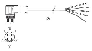
Figure 66: Adapter cable, e.g. part no. 2106174 (2 m)
