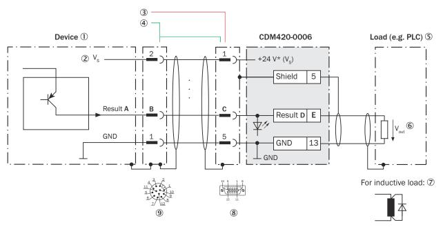
Figure 217: Wiring the "Result 1" and "Result 2" digital outputs of the device in the connection module CDM420-0006, Ethernet variant with male connector, M12, 12-pin, A-coded.
