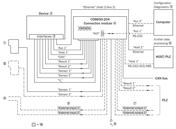
Figure 169: Connection of the device to peripherals via CDB650-204 (overview)
