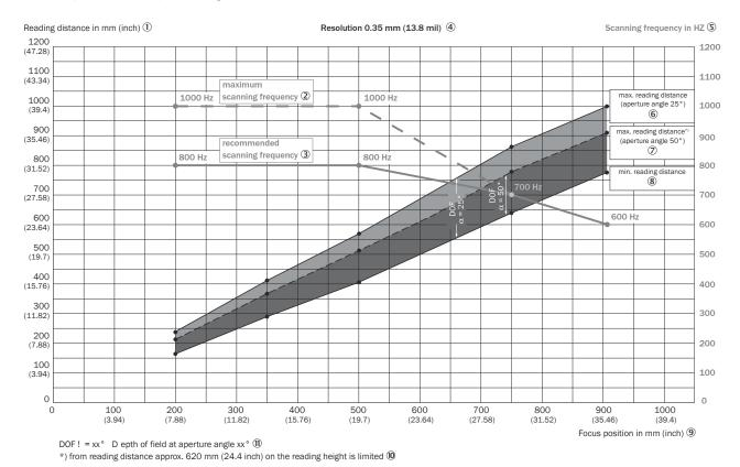
Depth of field ranges of the CLV650 line scanner with front reading window: Resolution 0.35 mm (13.8 mil)
