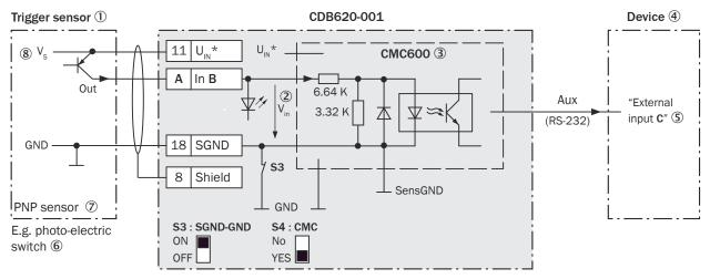
Figure 164: Trigger sensor supplied with power by connection module CDB620-001
