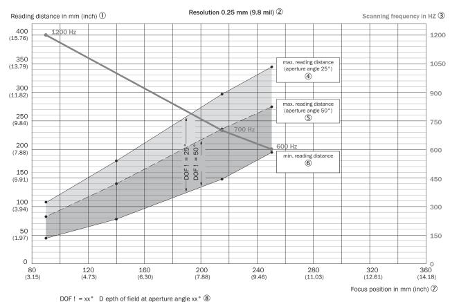
Figure 113: Depth of field ranges for CLV640-Xxx0, line (X = 2) or raster (X = 3), 0.25 mm resolution, glass viewing window, on the side. Minimum and maximum reading distance as a function of focus position and aperture angle
