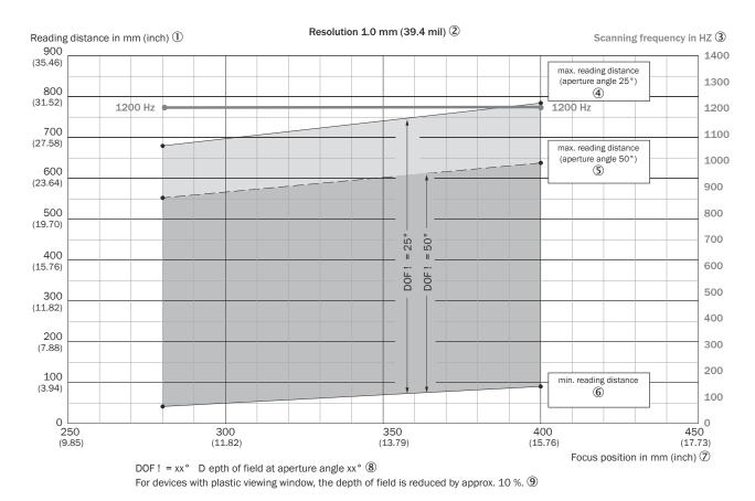
Figure 116: Depth of field ranges for CLV640-Xxx0, line (X = 2) or raster (X = 3), 1.00 mm resolution, glass viewing window, on the side. Minimum and maximum reading distance as a function of focus position and aperture angle
