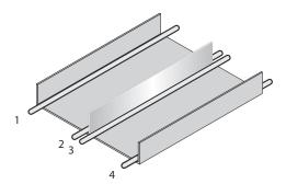
Figure 40: Alternative laying - Separate cables with metallic separators
