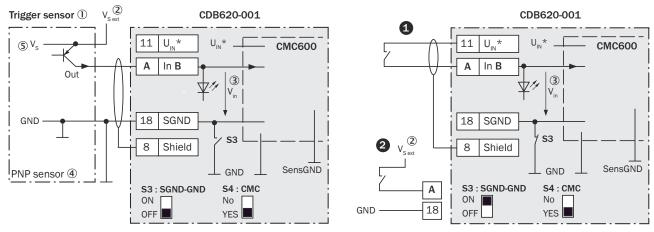
Figure 165: Left: Trigger sensor connected potential-free and supplied with power externally. Right: alternative switch, *1* supplied with power by connection module CDB620-001 or connected volt-free and supplied with power externally. Now select switch setting S3 as shown in the left figure.
