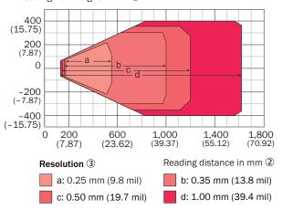
Figure 125: Reading field diagram for CLV650-Xxx0, standard density, line (X = 0), glass viewing window, at the front
