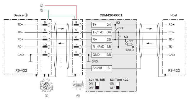
Figure 189: Wiring data interface RS-422 of the device in the CDM420-0001 connection module, Ethernet variant with male connector, M12, 17-pin, A-coded
