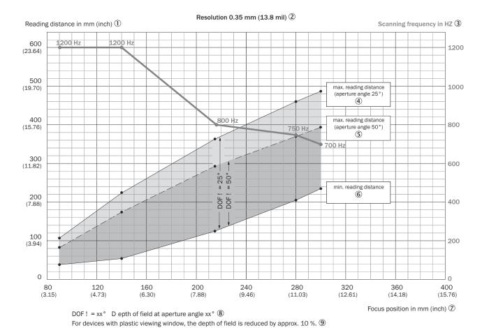
Figure 114: Depth of field ranges for CLV640-Xxx0, line (X = 2) or raster (X = 3), 0.35 mm resolution, glass viewing window, on the side. Minimum and maximum reading distance as a function of focus position and aperture angle
