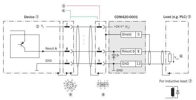
Figure 198: Wiring the digital outputs "Result 1" and "Result 2" of the device in the connection module CDM420-0001, Ethernet variant with male connector, M12, 12-pin, A-coded
