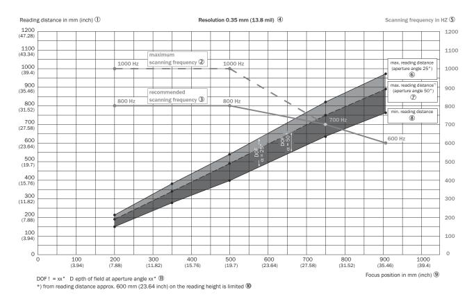
Depth of field ranges of the CLV650 line scanner with oscillating mirror: Resolution 0.35 mm (13.8 mil)
