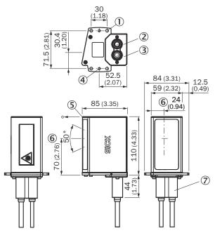
Figure 79: CLV62x/CLV63x/CLV64x: Ethernet variant in IP69K protective housing, with front viewing window and two M12 connections. structure and device dimensions, unit: mm (inch), decimal separator: period
