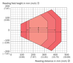
Devices with plastic viewing window (CLV631-xxx1): the depth of field is reduced by approx. 10 %. ③
