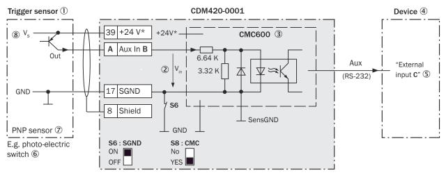
Figure 196: Trigger sensor supplied with power by connection module CDM420-0001
