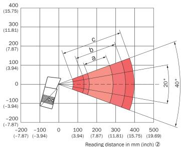
Devices with plastic viewing window (CLV640-6xx1): the depth of field is reduced by approx. 10 %. ③
