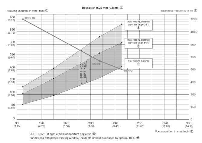
Figure 108: Depth of field ranges for CLV640-Xxx0, line (X = 0) or raster (X = 1), 0.25 mm resolution, glass viewing window, at the front. Minimum and maximum reading distance as a function of focus position and aperture angle
