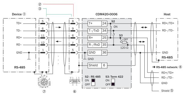
Figure 210: Wiring the RS-485 data interface of the device in the CDM420-0006 connection module, Ethernet variant with male connector, M12, 17-pin, A-coded.
