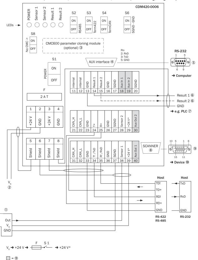
Device = CLV65x-xYxxxF0 (serial variant, Y=0 or Ethernet variant, Y = 1 or 8) with heating, 1 digital input used
