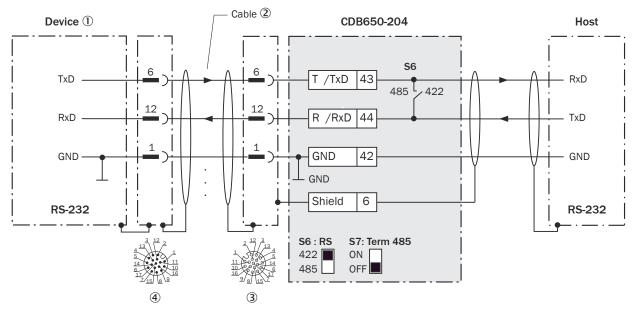
Figure 172: Wiring data interface RS-232 of the device in the connection module CDB650-204
