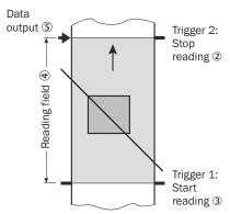
Figure 17: Start/Stop operating mode of the device in stand-alone operation
