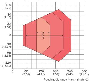
Devices with plastic viewing window (CLV632-6xx1): the depth of field is reduced by approx. 10 %. 3
