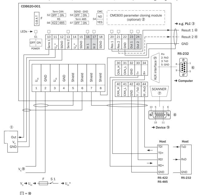
Device = CLV65x-xYxxxF0 (serial variant, Y=0 or Ethernet variant, Y = 1 or 8) with heating, 1 digital input used
