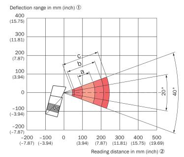
Devices with plastic viewing window (CLV632-6xx1): the depth of field is reduced by approx. 10 %. ③
