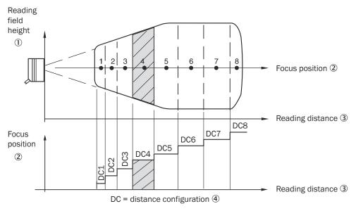
Figure 20: Focus switching: Division of the total reading range into distance configurations
