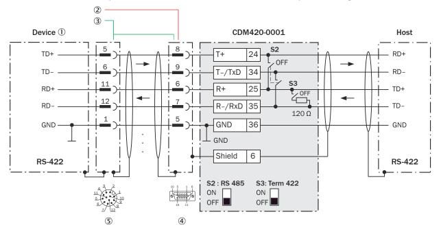
Figure 188: Wiring data interface RS-422 of the device in the CDM420-0001 connection module, Ethernet variant with male connector, M12, 12-pin, A-coded
