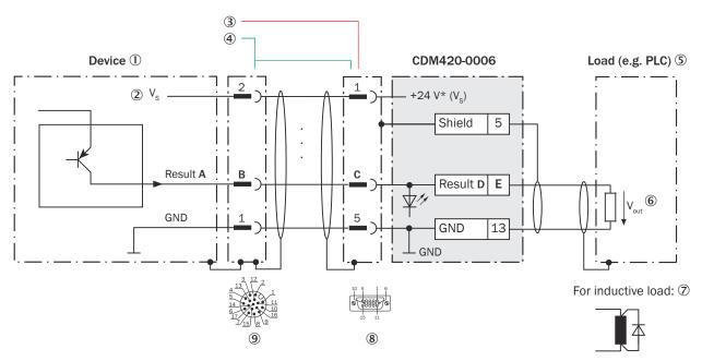
Figure 218: Wiring the digital outputs "Result 1" and "Result 2" of the device in the connection module CDM420-0006, Ethernet variant with male connector, M12, 17-pin, A-coded
