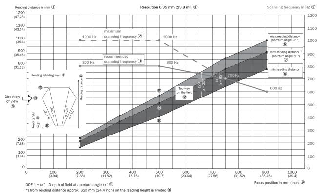
Figure 133: Meaning of the marks B, B and B in the reading field diagram D in relation to the depth of field diagram
