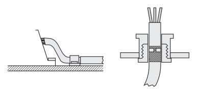
Figure 41: Shield connection in plastic housings
