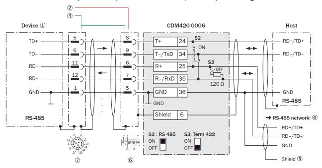
Figure 209: Wiring the RS-485 data interface of the device in the CDM420-0006 connection module, Ethernet variant with male connector, M12, 12-pin, A-coded.
