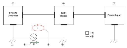
Figure 35: Example: Occurrence of equipotential bonding currents in the system configuration
