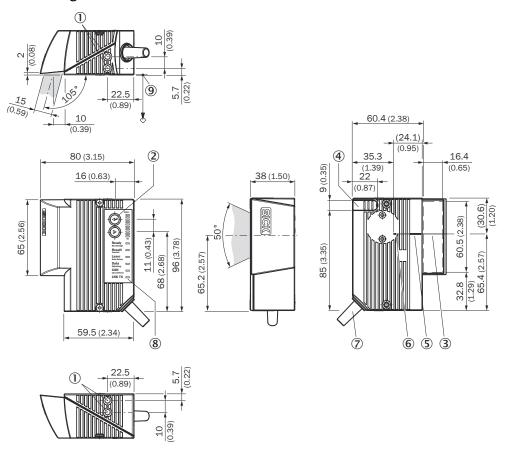
Figure 71: CLV63x to CLV65x: Serial variant in IP65 standard housing, with side viewing window and connecting cable. structure and device dimensions, unit: mm (inch), decimal separator: period
