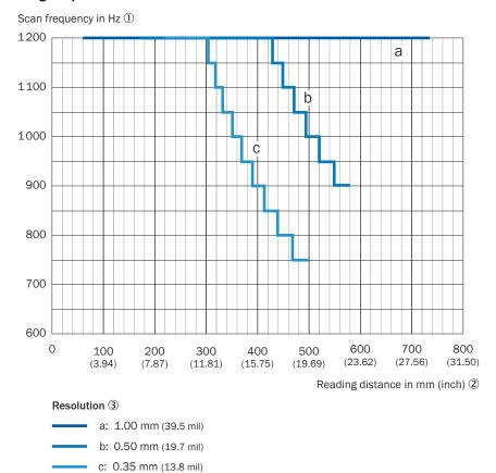
Figure 87: All sensor types: Scanning frequency characteristic curve field for CLV630-xxxx, Long Range, viewing window at the front
