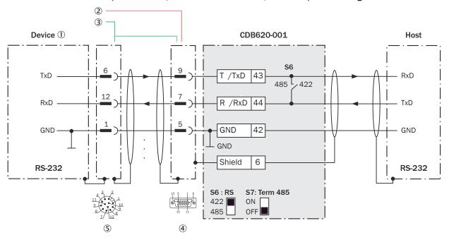
Figure 154: Wiring data interface RS-232 of the device in the CDB620-001 connection module, Ethernet variant with male connector, M12, 12-pin, A-coded
