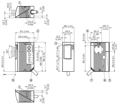
Figure 70: CLV63x to CLV65x: Serial variant in standard housing, with front viewing window and connecting cable. structure and device dimensions, unit: mm (inch), decimal separator: period
