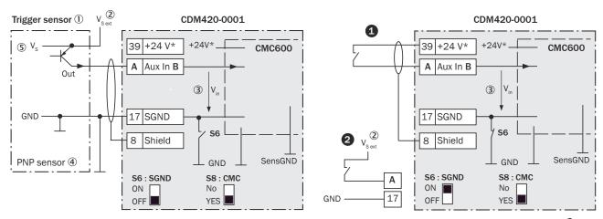
Figure 197: Left: Trigger sensor connected potential-free and supplied with power externally. Right: Alternatively switch, *1* supplied with power by connection module CDM420-0001 or @connected potential-free and supplied with power externally. Switch setting S3 then as in left figure.
