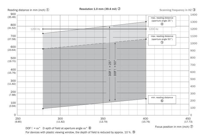
Figure 111: Depth of field ranges for CLV640-Xxx0, line (X = 0) or raster (X = 1), 1.00 mm resolution, glass viewing window, at the front. Minimum and maximum reading distance as a function of focus position and aperture angle
