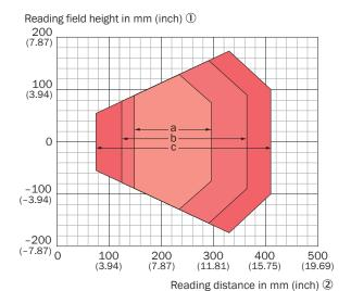
Devices with plastic viewing window (CLV631-xxx1): the depth of field is reduced by approx. 10 %. 3
