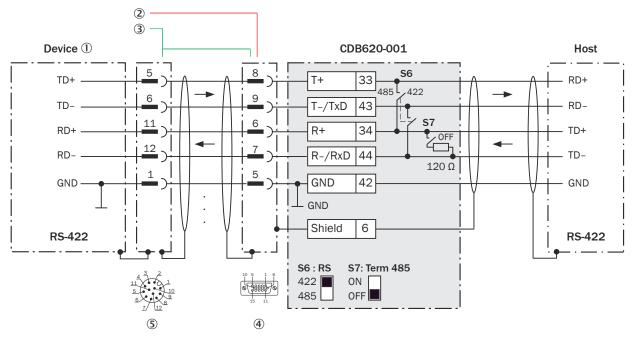
Figure 156: Wiring data interface RS-422 of the device in the CDB620-001 connection module, Ethernet variant with male connector, M12, 12-pin, A-coded
