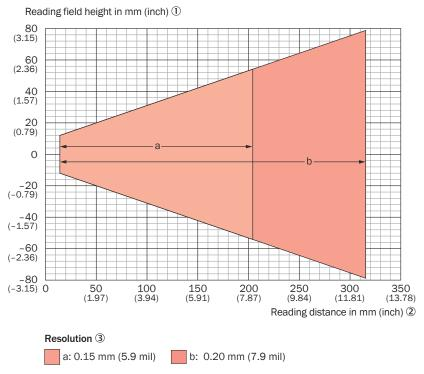
Figure 105: Reading field diagram for CLV642-Xxx0, High resolution, line (X = 2), glass viewing window, on the side
