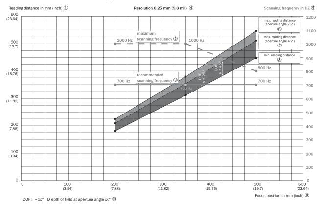
Depth of field ranges of the CLV650 line scanner with reading window: Resolution 0.25 mm (9.8 mil)
