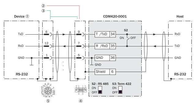
Figure 187: Wiring data interface RS-232 of the device in the CDM420-0001 connection module, Ethernet variant with male connector, M12, 17-pin, A-coded
