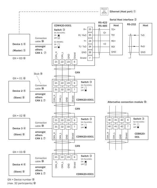
Figure 192: Wire the CAN interface of the device in the CDM420-0001 connection module. Connection and looping through of the supply voltage and connection of a trigger sensor for read cycle generation at the master, for example, are disregarded here!
