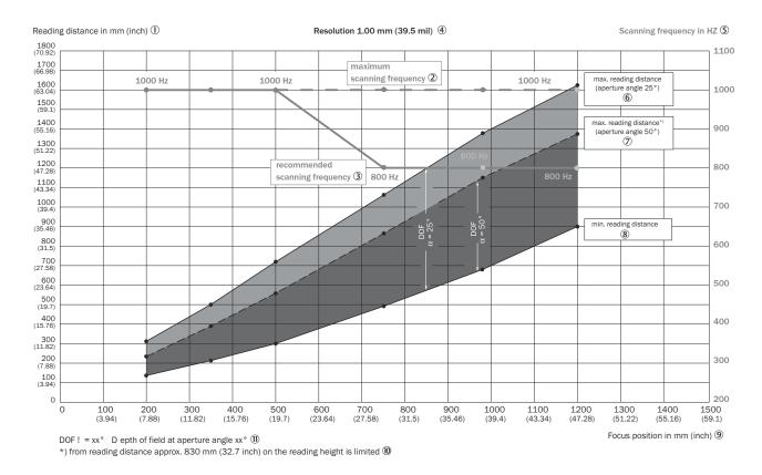
Depth of field ranges of the CLV650 line scanner with front reading window: Resolution 1.00 mm (39.5 mil)
