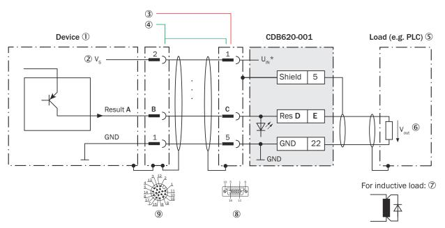
Figure 167: Wiring the "Result 1" and "Result 2" digital outputs of the device in the connection module CDB620-001, Ethernet variant with male connector, M12, 17-pin, A-coded.
