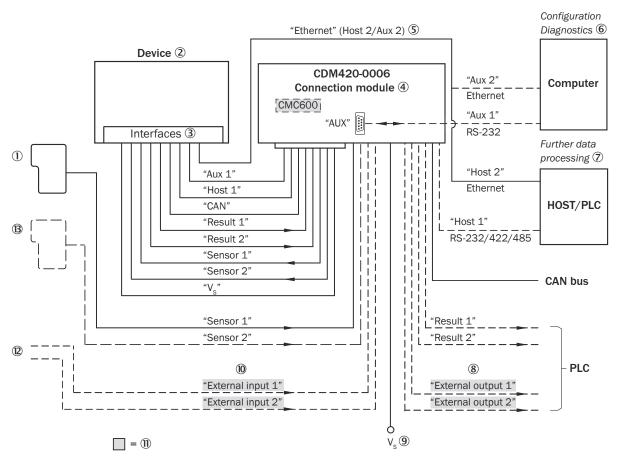
Figure 201: Connection of the device to peripherals via CDM420-0006 (overview)
