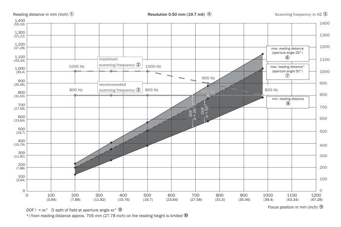
Depth of field ranges of the CLV650 line scanner with oscillating mirror: Resolution 0.50 mm (19.7 mil)
