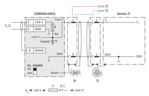
Figure 185: Connecting supply voltage for the device in the CDM420-0001 connection module, Ethernet variant with male connector, M12, 17-pin, A-coded
