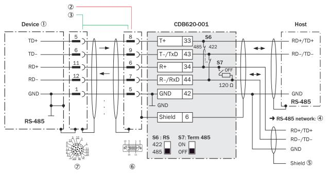
Figure 159: Wiring the RS-485 data interface of the device in the CDB620-001 connection module, Ethernet variant with male connector, M12, 17-pin, A-coded
