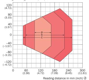
Devices with plastic viewing window (CLV632-xxx1): the depth of field is reduced by approx. 10 %. ③
