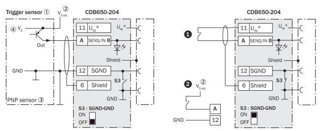
Figure 177: Left: Trigger sensor connected potential-free and supplied with power externally. Right: Alternatively switch, *1* supplied with power by connection module CDB650-204 or 2 connected potential-free and supplied with power externally. Now select switch setting S3 as shown in the left figure.
