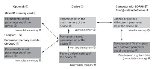
Figure 54: Configuration with SOPAS ET and saving the parameter set
