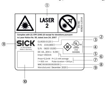
Figure 5: CLV63x, CLV64x and CLV65x: Example of type label for CLV630-0120 (serial variant). For devices in IP65 standard housing. Electrical values shown here for devices without heating. Figure may differ.
