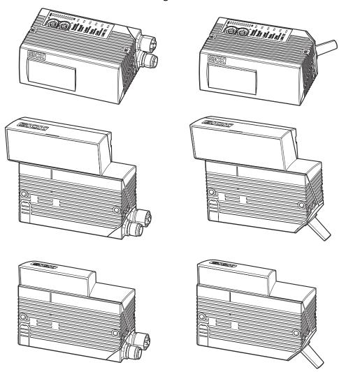
Figure 9: Device variants without heating (from top to bottom): Housing shape with front viewing window, with oscillating mirror and side viewing window, and with only side viewing window. All types with swivel connector (Ethernet variant, shown on left) or with cable connection (serial variant, shown on right).
