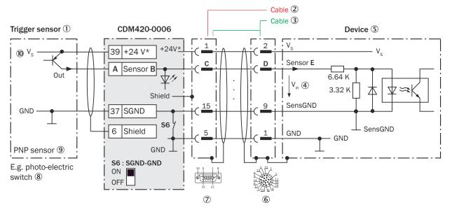
Figure 213: Trigger sensor supplied with power by connection module CDM420-0006, Ethernet variant with male connector, M12, 17-pin, A-coded
