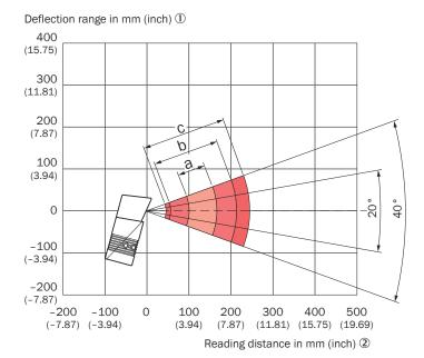
Devices with plastic viewing window (CLV640-6xx1): the depth of field is reduced by approx. 10 %. ③
