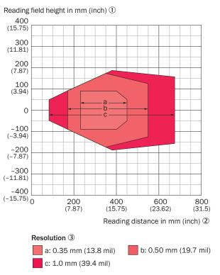
Figure 82: Reading field diagram for CLV630-Xxx1S01, long range, line scanner (X = 0) or raster scanner (X = 1), plastic viewing window, at the front, oval light spot
