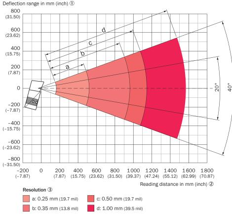
Figure 128: Oscillating mirror deflection width diagram for CLV650-6xx0, standard density, line with oscillating mirror, glass viewing window, on the side
