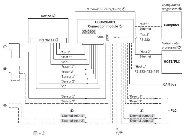
Figure 150: Connection of the device to peripherals via CDB620-001 (overview)
