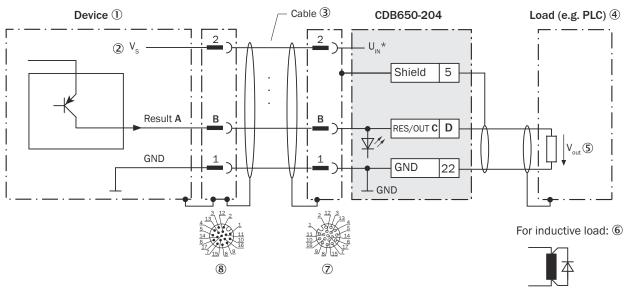
Figure 180: Wiring the digital outputs "Result 1" and "Result 2" of the device in the connection module CDB650-204
