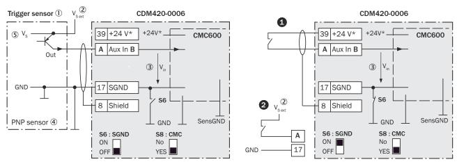
Figure 216: Left: Trigger sensor connected potential-free and supplied with power externally. Right: Alternatively switch, *1* supplied with power by connection module CDM420-0006 or @connected potential-free and supplied with power externally. Switch setting S3 then as in left figure.
