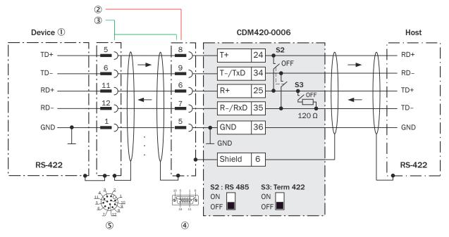
Figure 207: Wiring data interface RS-422 of the device in the CDM420-0006 connection module, Ethernet variant with male connector, M12, 12-pin, A-coded
