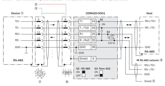
Figure 190: Wiring data interface RS-485 of the device in the CDM420-0001 connection module, Ethernet variant with male connector, M12, 12-pin, A-coded
