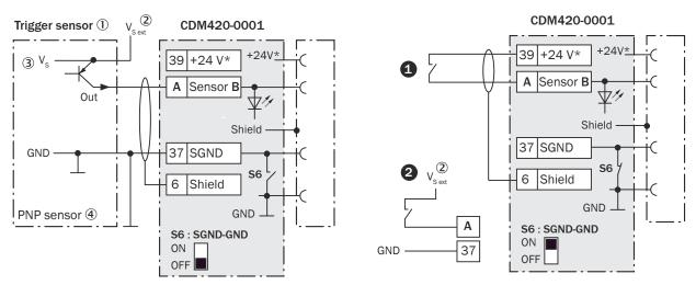
Figure 195: Left: Trigger sensor connected potential-free and supplied with power externally. Right: alternative switch, *1* supplied with power by connection module CDM420-0001 or @connected volt-free and supplied with power externally. Now select switch setting S6 as shown in the left figure.
