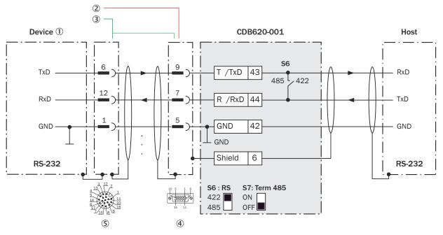
Figure 155: Wiring data interface RS-232 of the device in the CDB620-001 connection module, Ethernet variant with male connector, M12, 17-pin, A-coded
