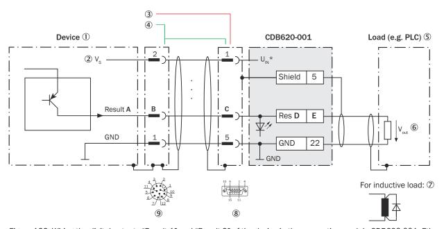
Figure 166: Wiring the digital outputs "Result 1" and "Result 2" of the device in the connection module CDB620-001, Ethernet variant with male connector, M12, 12-pin, A-coded
