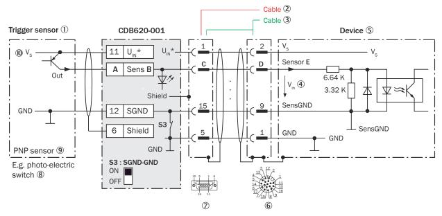
Figure 162: Trigger sensor supplied with power by connection module CDB620-001, Ethernet variant with male connector, M12, 17-pin, A-coded
