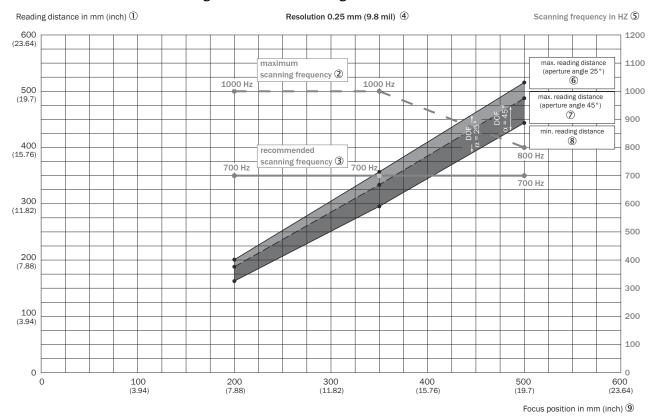
Depth of field ranges of the CLV650 line scanner with oscillating mirror (side reading window: Resolution 0.25 mm (9.8 mil); aperture angle 25°/45°
