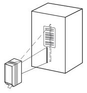
Figure 56: Appearance of the scan line in "Adjusting Mode"
