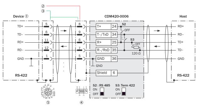
Figure 208: Wiring data interface RS-422 of the device in the CDM420-0006 connection module, Ethernet variant with male connector, M12, 17-pin, A-coded
