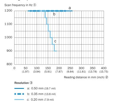
Figure 97: All sensor types: Scanning frequency characteristic curve field for CLV632-xxxx, Short Range, viewing window at the front
