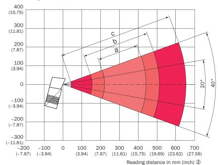
Devices with plastic viewing window (CLV640-6xx1): the depth of field is reduced by approx. 10 %. ③
