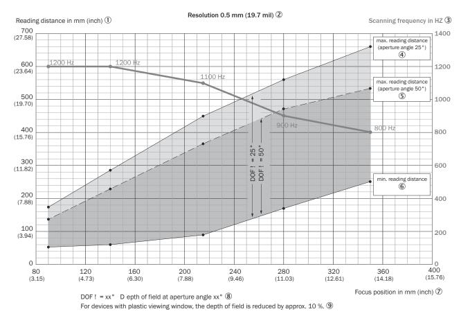
Figure 110: Depth of field ranges for CLV640-Xxx0, line (X = 0) or raster (X = 1), 0.50 mm standard resolution, glass viewing window, at the front. Minimum and maximum reading distance as a function of focus position and aperture angle
