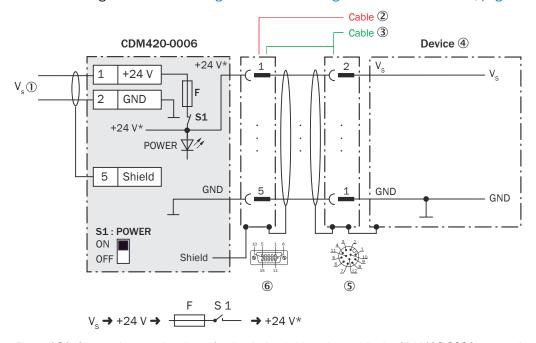
Figure 203: Connecting supply voltage for the device (without heater) in the CDM420-0006 connection module, Ethernet variant with male connector, M12, 12-pin, A-coded
