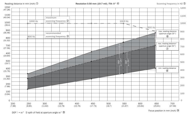
\*) from reading distance approx. 645 mm (25.4 inch) on the reading height is limited 10
