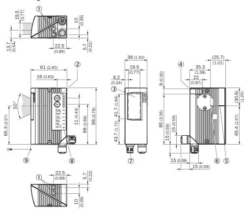
Figure 67: CLV63x to CLV65x: Ethernet variant in standard housing, with front viewing window and swivel connector. structure and device dimensions, unit: mm (inch), decimal separator: period
