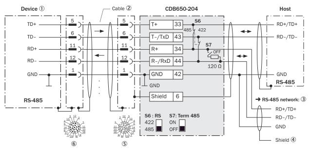
Figure 174: Wiring data interface RS-485 of the device in connection module CDB650-204.
