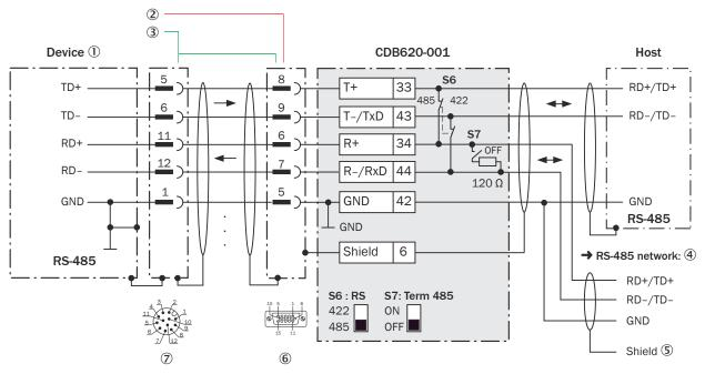
Figure 158: Wiring data interface RS-485 of the device in the CDB620-001 connection module, Ethernet variant with male connector, M12, 12-pin, A-coded
