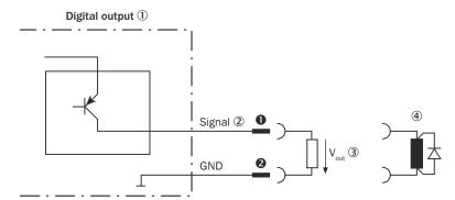
Figure 53: Wiring a digital output on the device
