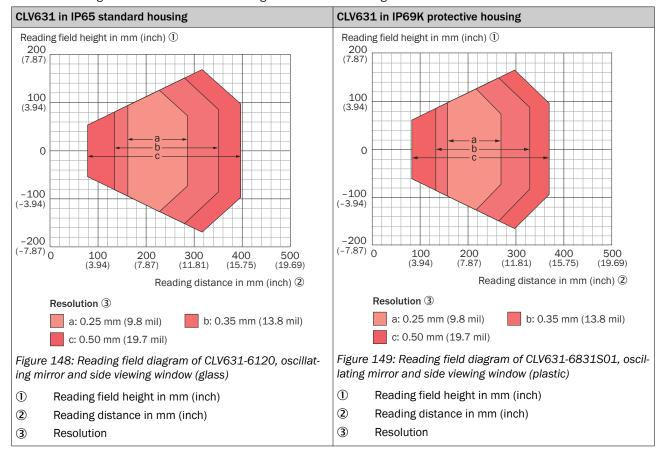
Table 35: Reading fields of CLV631 with oscillating mirror and side viewing window
