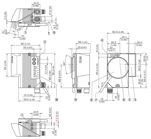
Figure 74: CLV63x to CLV65x: Ethernet variant in standard housing, with external heating, side viewing window and swivel connector. structure and device dimensions, unit: mm (inch), decimal separator: period
