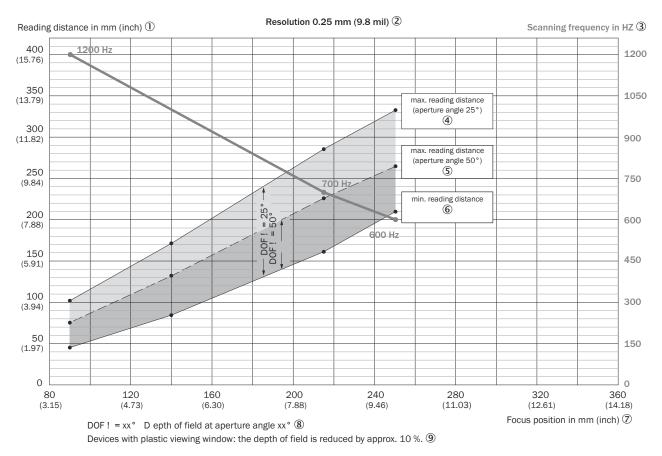
Figure 118: Depth of field ranges for CLV640-6xx0, 0.25 mm resolution, oscillating mirror, glass viewing window, on the side. Minimum and maximum reading distance as a function of focus position and aperture angle
