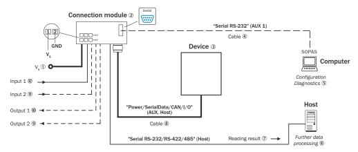
Figure 16: CLV63x to CLV65x facilities for connecting, serial variant
