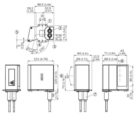
Figure 80: CLV63x / CLV64x: Ethernet variant in IP69K protective housing, with oscillating mirror (side viewing window) and two M12 connections. structure and device dimensions, unit: mm (inch), decimal separator: period
