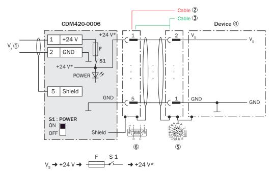
Figure 204: Connecting supply voltage for the device (without heater) in the CDM420-0006 connection module, Ethernet variant with male connector, M12, 17-pin, A-coded
