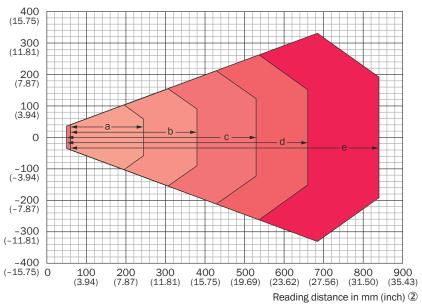
For devices with plastic reading window (CLV640-0831S01): the depth of field is reduced by approx. 10 %. ③
