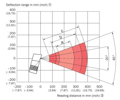
Devices with plastic viewing window (CLV631-6xx1): the depth of field is reduced by approx. 10 %. 3
