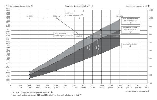
Depth of field ranges of the CLV650 line scanner with oscillating mirror: Resolution 1.00 mm (39.5 mil)
