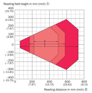
Devices with plastic viewing window (CLV630-xxx1): the depth of field is reduced by approx. 10 %. ③
