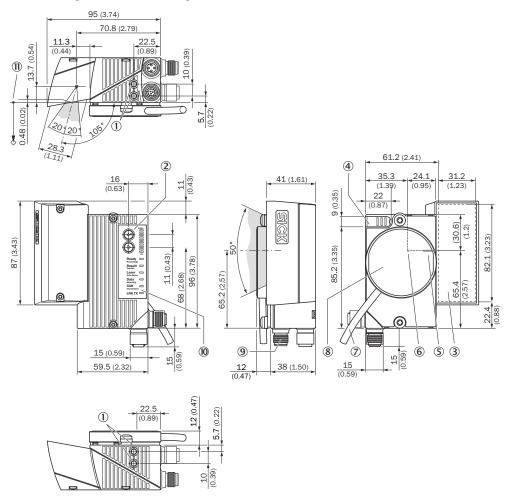
Figure 75: CLV63x to CLV65x: Ethernet variant in standard housing, with external heating, oscillating mirror (side viewing window) and swivel connector. structure and device dimensions, unit: mm (inch), decimal separator: period
