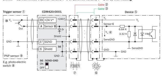
Figure 193: Trigger sensor supplied with power by connection module CDM420-0001, Ethernet variant with male connector, M12, 12-pin, A-coded
