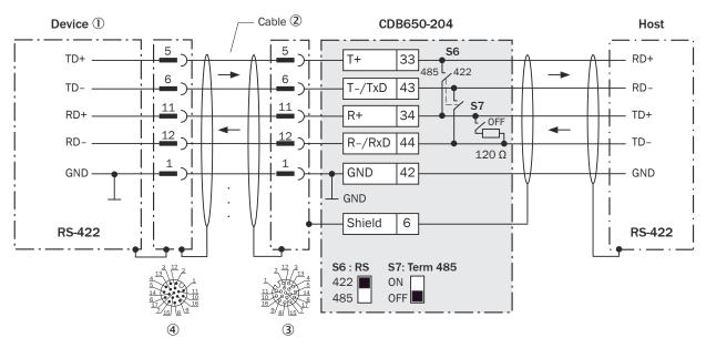
Figure 173: Wiring data interface RS-422 of the device in the connection module CDB650-204
