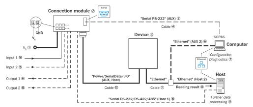
Figure 15: Connection options for CLV63x to CLV65x, Ethernet variant (male connector, M12, 17-pin, A-coded)
