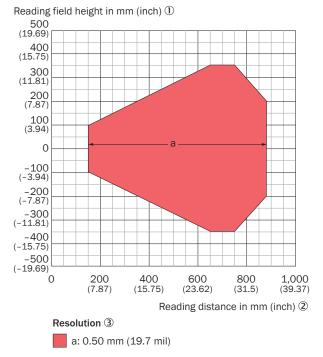
Figure 131: Reading field diagram for CLV651-6xx0, low density, line with oscillating mirror, glass viewing window, on the side
