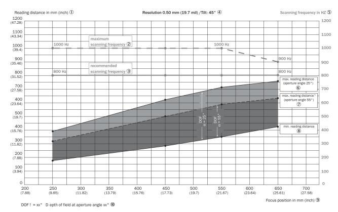
Depth of field ranges of the CLV651 line scanner with front reading window: Resolution 0.5 mm (19.7 mil); inclination angle  $45^{\circ}$ ; aperture angle  $25^{\circ}/55^{\circ}$
