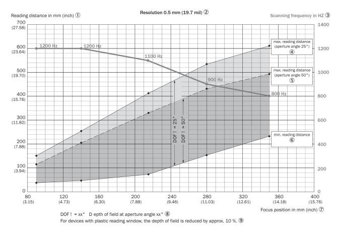
Figure 115: Depth of field ranges for CLV640-Xxx0, line (X = 2) or raster (X = 3), 0.50 mm standard resolution, glass viewing window, on the side. Minimum and maximum reading distance as a function of focus position and aperture angle
