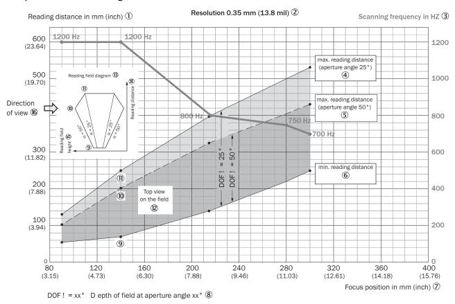
Figure 106: Meaning of the marks @, @ and @ in the reading field diagram @ in relation to the depth of field diagram
