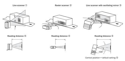
Figure 24: Allocation of scan line(s) to bar code and conveyor direction
