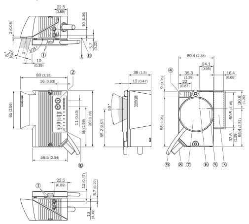
Figure 77: CLV63x to CLV65x: Serial variant in standard housing with external heating, side viewing window and connecting cable. structure and device dimensions, unit: mm (inch), decimal separator: period
