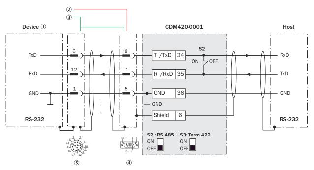
Figure 186: Wiring data interface RS-232 of the device in the CDM420-0001 connection module, Ethernet variant with male connector, M12, 12-pin, A-coded
