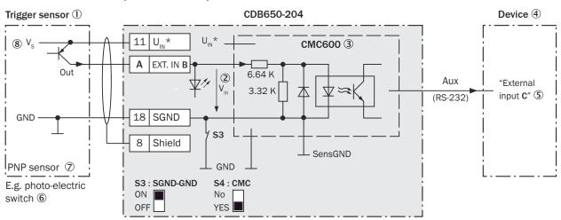
Figure 178: Trigger sensor supplied with power by connection module CDB650-204
