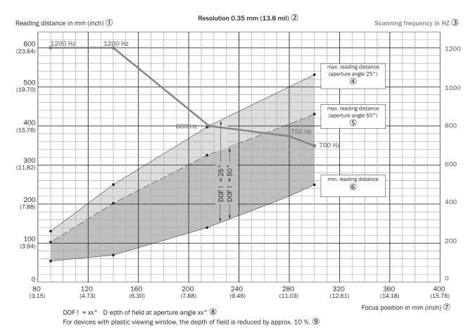
Figure 109: Depth of field ranges for CLV640-Xxx0, line (X = 0) or raster (X = 1), 0.35 mm resolution, glass viewing window, at the front. Minimum and maximum reading distance as a function of focus position and aperture angle
