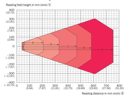
For devices with plastic reading window (CLV640-6120S01,CLV640-6831S01 and CLV640-6121S01): the depth of field is reduced by approx. 10 %. 3
