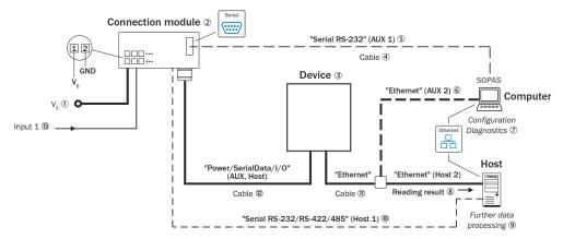
Figure 14: Connection options for CLV63x to CLV65x, Ethernet variant (male connector, M12, 12-pin, A-coded)
