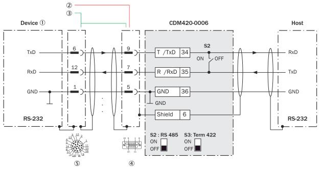
Figure 206: Wiring data interface RS-232 of the device in the CDM420-0006 connection module, Ethernet variant with male connector, M12, 17-pin, A-coded
