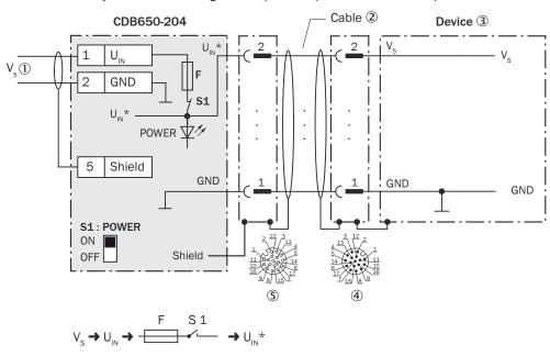
Figure 171: Connecting supply voltage for the device in CDB650-204 connection module.
