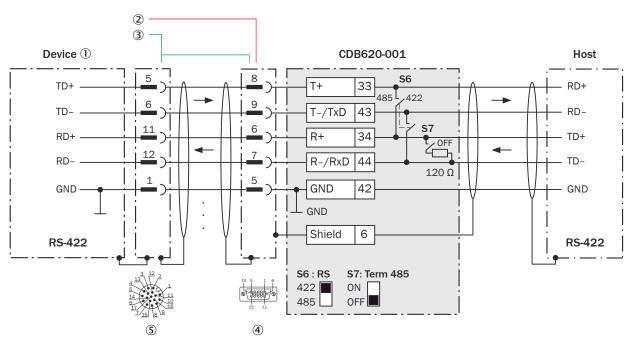
Figure 157: Wiring data interface RS-422 of the device in the CDB620-001 connection module, Ethernet variant with male connector, M12, 17-pin, A-coded
