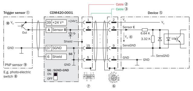
Figure 194: Trigger sensor supplied with power by connection module CDM420-0001, Ethernet variant with male connector, M12, 17-pin, A-coded
