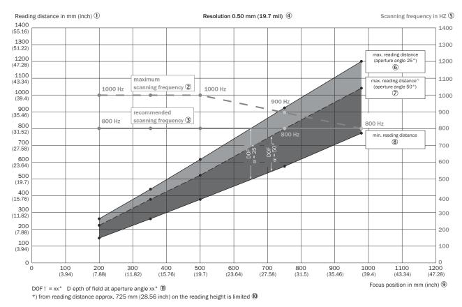
Depth of field ranges of the CLV650 line scanner with front reading window: Resolution 0.50 mm (19.7 mil)
