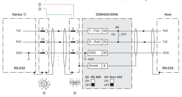
Figure 205: Wiring data interface RS-232 of the device in the CDM420-0006 connection module, Ethernet variant with male connector, M12, 12-pin, A-coded
