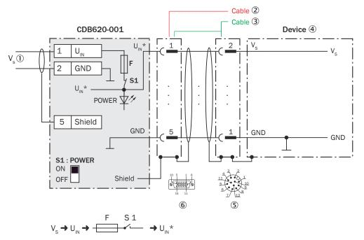
Figure 152: Connecting supply voltage for the device in the CDB620-001 connection module, Ethernet variant with male connector, M12, 12-pin, A-coded
