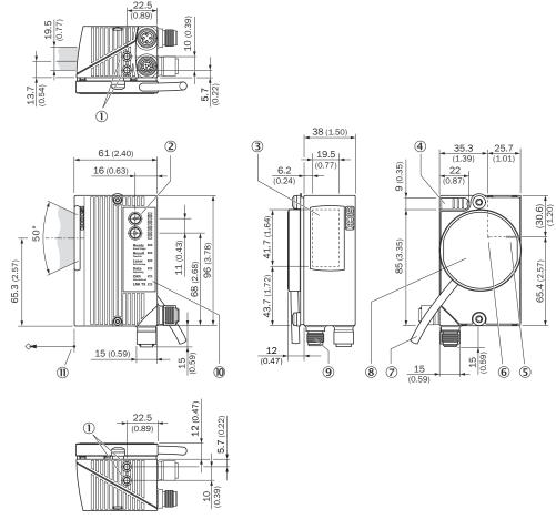
Figure 73: CLV63x to CLV65x: Ethernet variant in standard housing, with external heating, front viewing window and swivel connector. structure and device dimensions, unit: mm (inch), decimal separator: period
