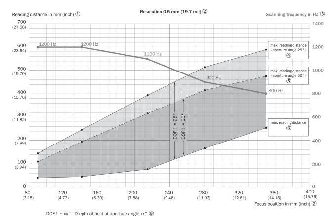
Devices with plastic viewing window: the depth of field is reduced by approx. 10 %. 9
