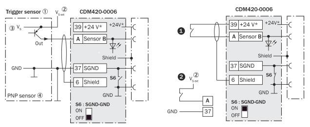
Figure 214: Left: Trigger sensor connected potential-free and supplied with power externally. Right: alternative switch, **0** supplied with power by connection module CDM420-0006 or **2** connected volt-free and supplied with power externally. Now select switch setting S6 as shown in the left figure.
