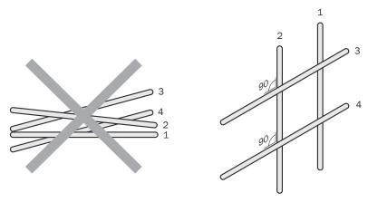
Figure 38: Cross cables at right angles
