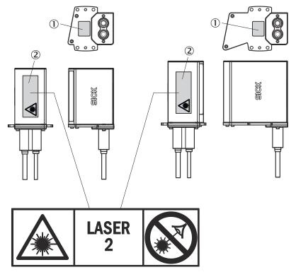
Figure 4: IP69K protective housing: Position and content of the laser warning label on the device
